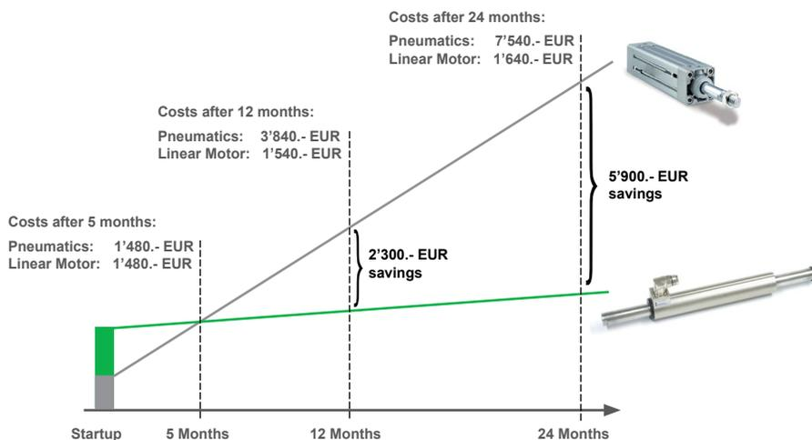
Analysis of the investment and energy costs in this application example shows that the savings from the use of an industrial linear motor, compared to the use of a pneumatic cylinder, are 2'300.- EUR and 5'900.- EUR at 12 and 24 months of service respectively.
